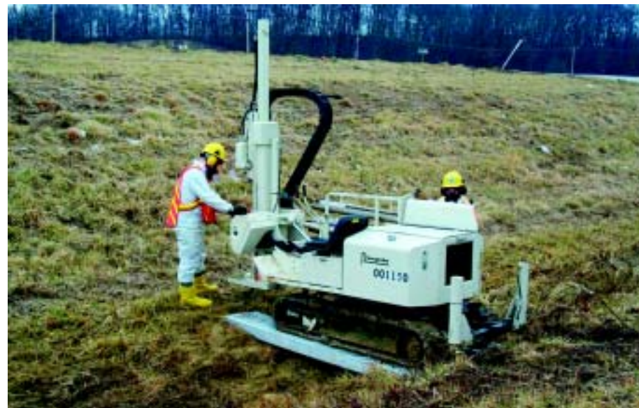
Staff conduct depth-discrete soil sampling using the Geoprobe® during a collaborative effort between the Missouri Department of Transportation and the Missouri Department of Natural Resources in determining the presence of hazardous chemicals.
