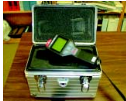
Staff use the radioactive isotope identifier during air monitoring.
