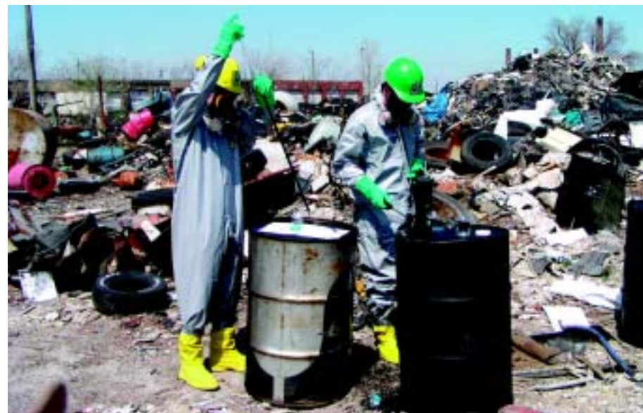
Staff sample the contents of drums to determine whether the contents are hazardous waste.
