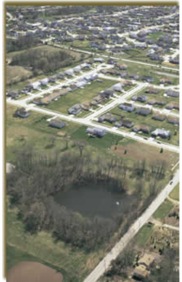
The Old Jamestown area in northern St. Louis County is a karst area prone to sinkholes, such as the one filled with water in the foreground. DNR photo by Nick Decker
