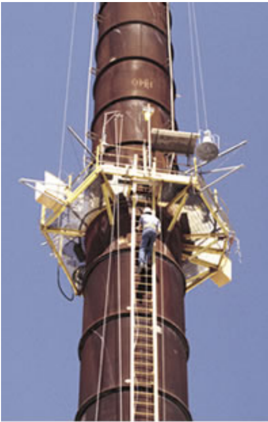
A stack testing engineer climbs to a testing platform at Chemical Lime in Ste. Genevieve to test plant emissions for particulate matter, sulfur dioxide, nitrogen oxides, and carbon monoxide. DNR photo by Doug Elley
