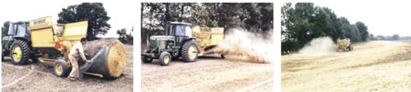
The large-bale power mulcher is one of the most commonly rented pieces of equipment that the Monroe County Soil and Water Conservation District has available. The mulcher allows farmers and contractors to cover a large area of freshly seeded ground with mulch and greatly reduce the threat of erosion. Kent Dye, of Paris, prepares a bale to load into the power mulcher.
