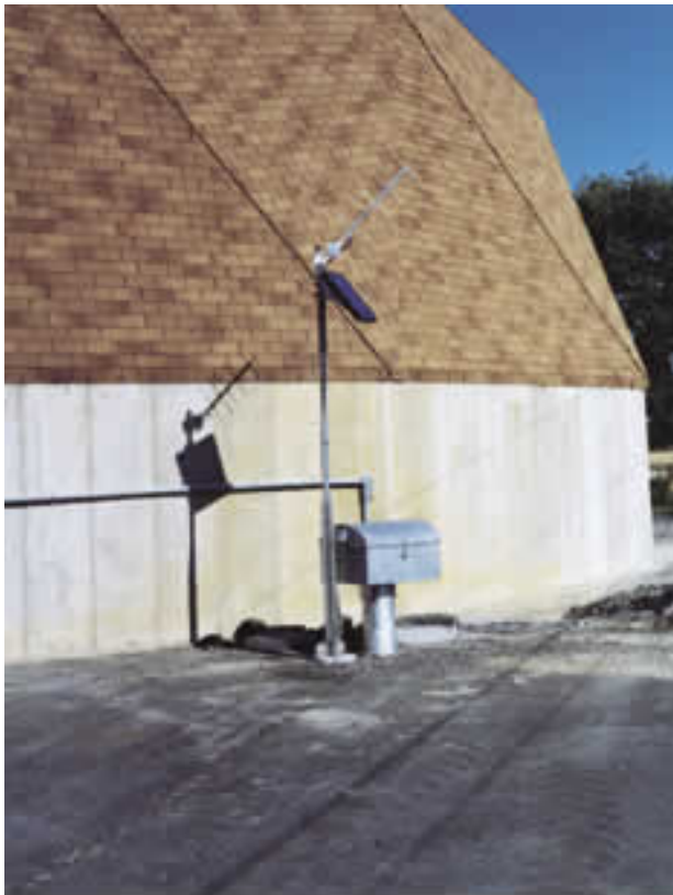
One of 70 groundwater monitoring stations across Missouri returns data via satellite every four hours. The data is available on the department's Web site at www.dnr.mo.gov/water.htm . DNR photo by Jim Vandike
