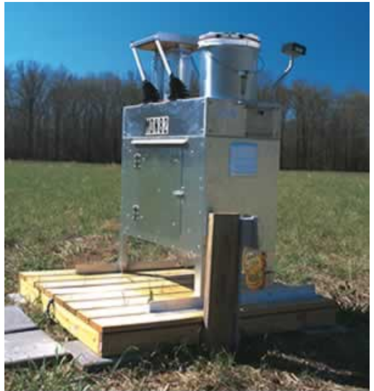
The Department of Natural Resources recently installed a rainfall monitoring station at Mingo National Wildlife Refuge near Puxico. The data gathered will be combined with that from other locations in the Mercury Deposition Network and will be used to monitor mercury levels in precipitation across North America.
