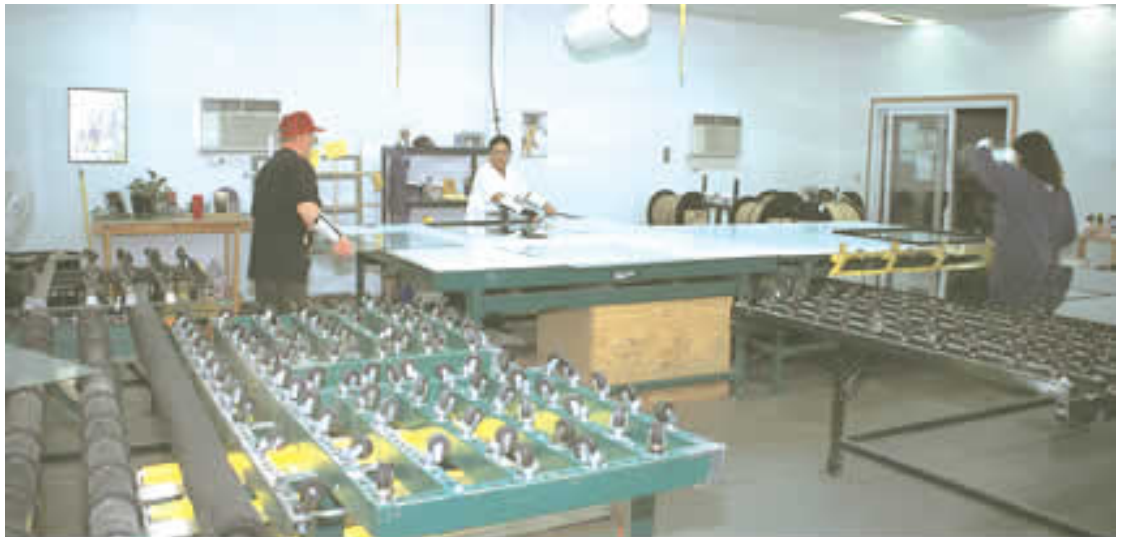
At Target Windows and Doors, employees prepare sheets of glass that will be made into Energy Star rated windows. In the finished windows, each pane is made of two sheets of glass separated by a gasket. The space in between is filled with inert argon gas which acts as insulation. The resulting windows are much more efficient than older, single-pane windows. DNR photo by Scott Myers
