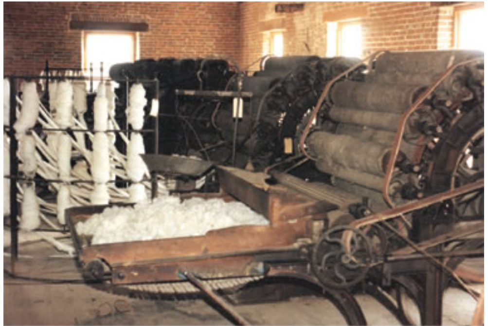
Vintage textile equipment, such as these carding engines, is on display inside the mill. DNR file photo.
