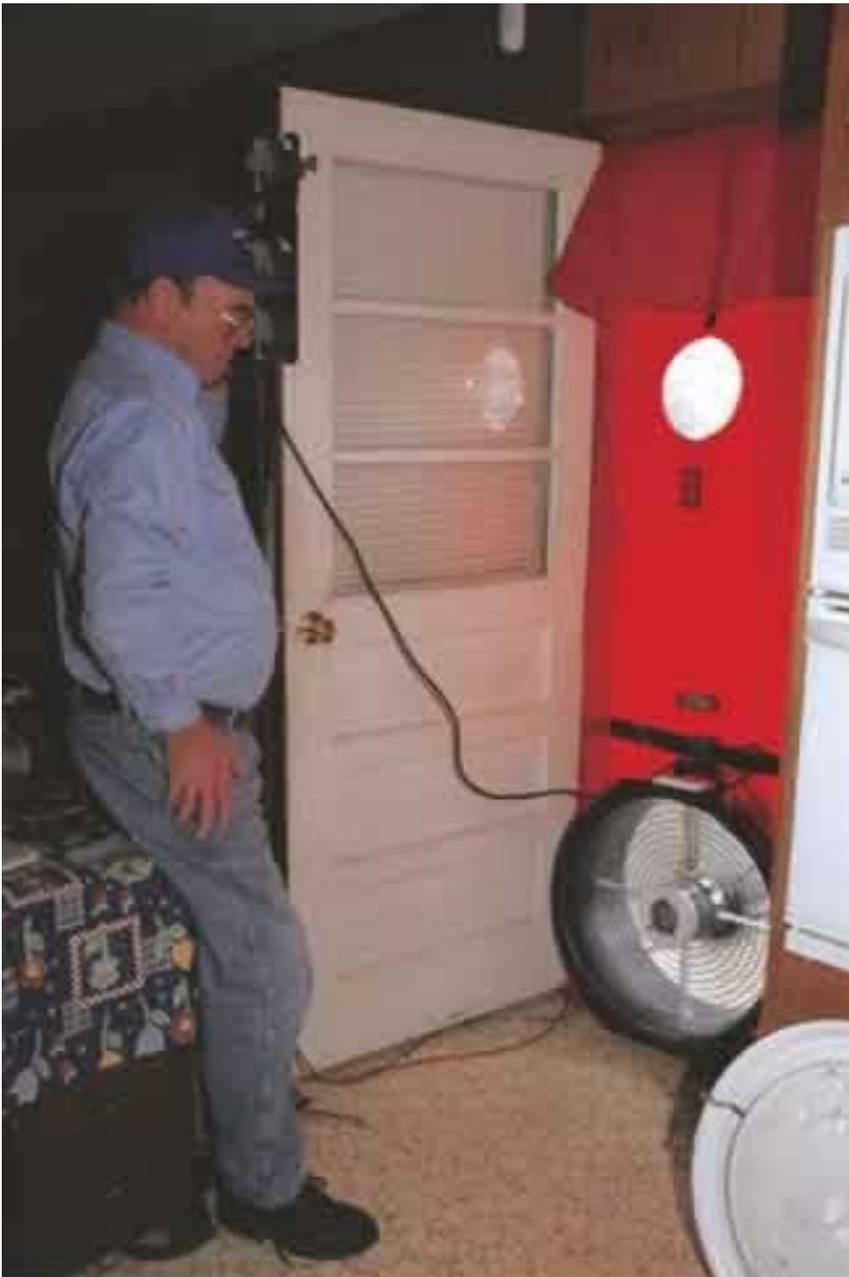
Skip Sears of Missouri Ozarks Community Action (MOCA) uses a blower door and fan to detect air leaks in a house being weatherized.
