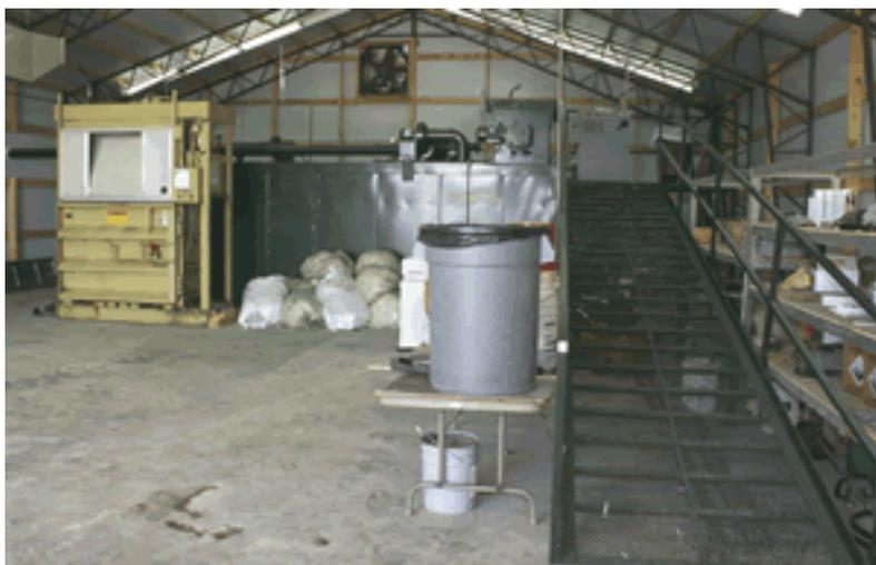
Bags of shredded paper will be placed in the in-vessel composting system at Reeds Spring High School. To the left of the bags is a cardboard compactor.
