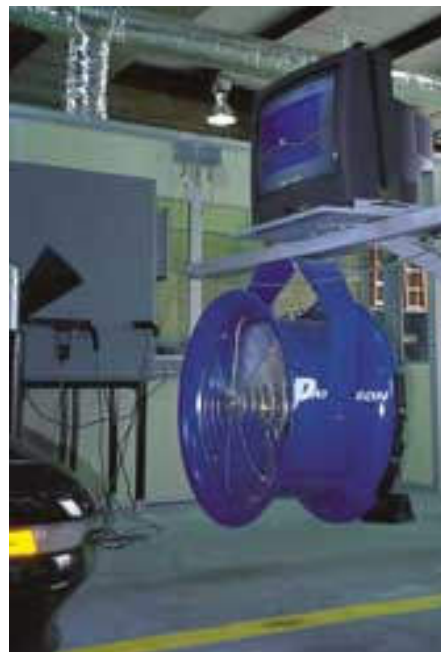
Along with the monitor that charts and tracks the treadmill emissions test, a powerful fan provides the air needed to keep the engine cool.
