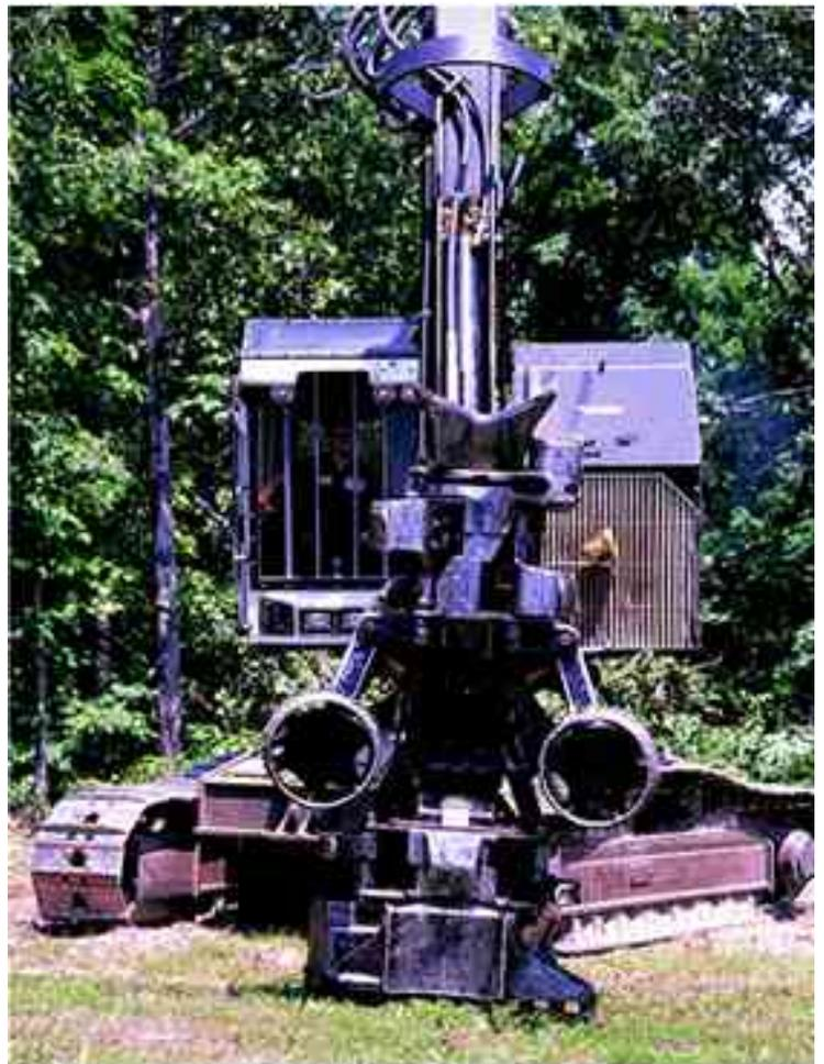
Modern timber-harvesting practices include the use of machinery such as this feller-buncher. From inside the cab, an operator maneuvers the machine into the forest where it slices off trees at the ground and strips their limbs. The bare stems are then loaded into the back of a truck for transport to a chipper. DNR photo by Nick Decker.
