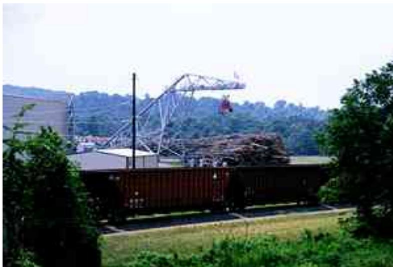
At the Willamette chip mill, a crane is used to move logs from truck to chipper. The wood chips then are loaded into railroad cars.
