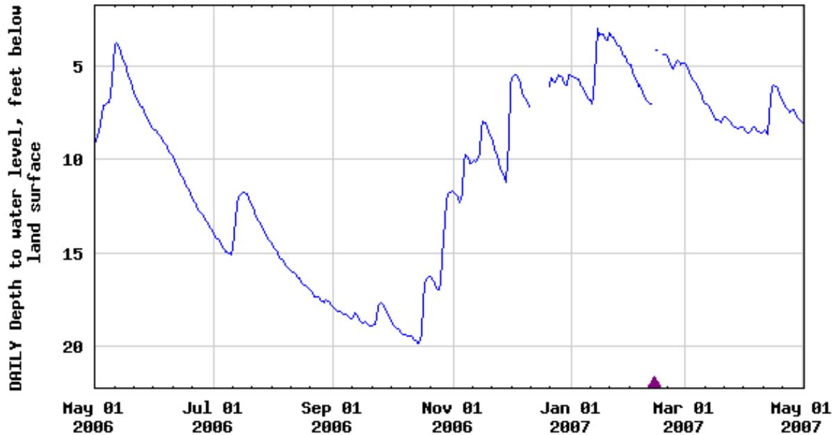
Figure 2. Daily hydrograph of Big Spring observation well showing recharge and discharge.
