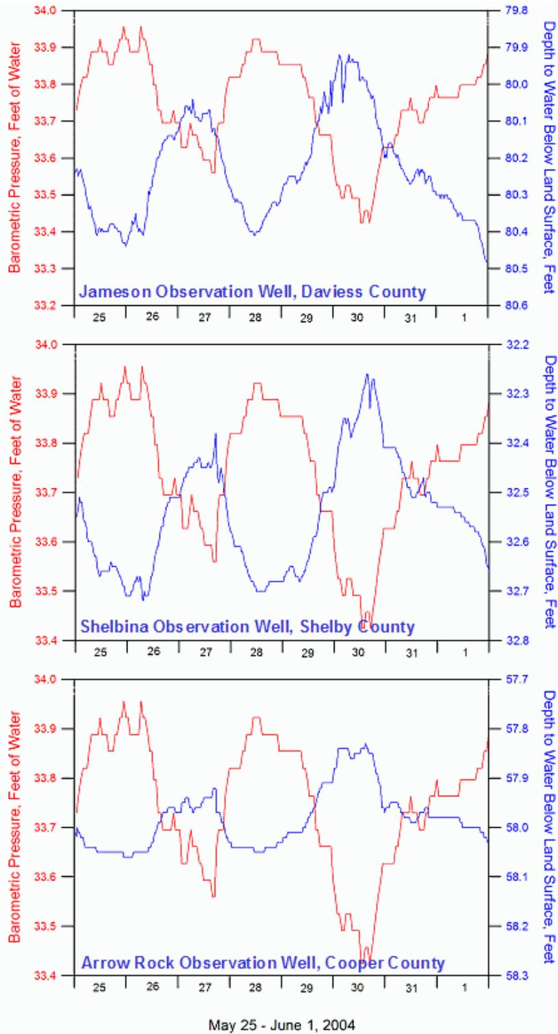
Figure 9. Hydrographs of Jameson, Shelbina, and Arrow Rock observation wells (blue) and barometric pressure at Sanborn Field, University of Missouri-Columbia (red) showing the effects of barometric pressure changes on groundwater levels.
