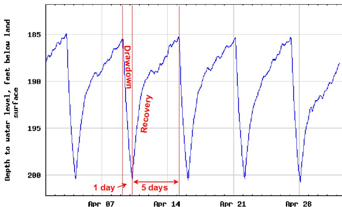
Figure 5. Water-level changes due to a nearby pumping well, Ramada Inn (Rolla) observation well
