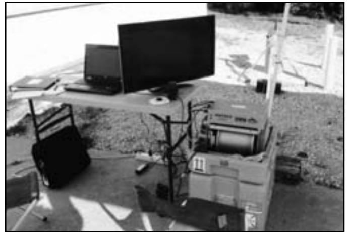
Cement bond logging equipment at the McCracken Core Library and Research Center.
