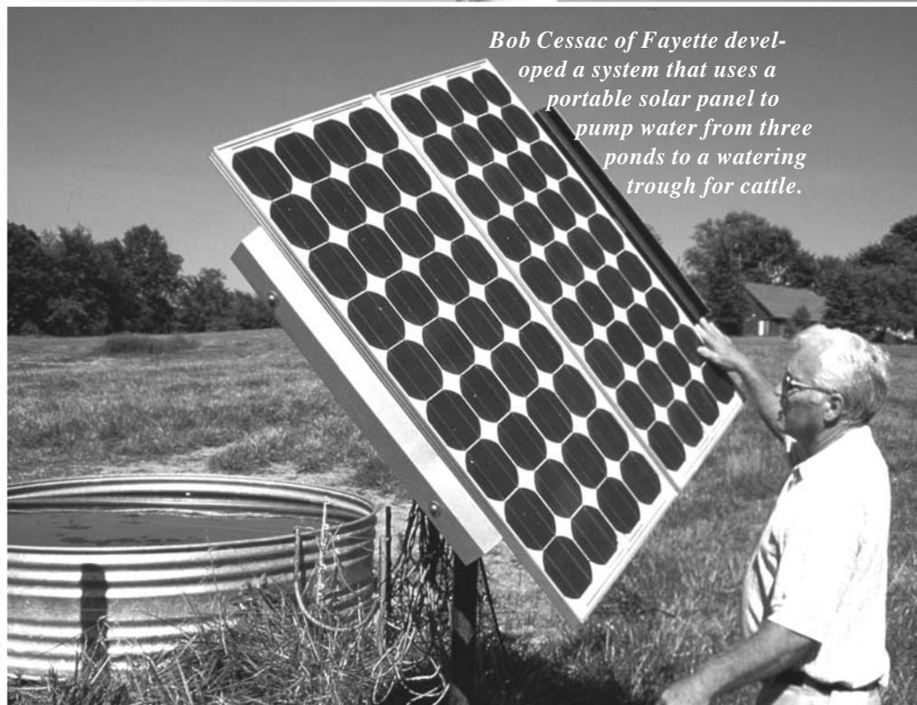
*Bob Cessac of Fayette developed a system that uses a portable solar panel to pump water from three ponds to a watering trough for cattle.*
