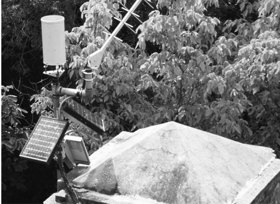
*Most of the U.S. Geological Survey's 105 stream-flow gauging stations, like this one on the Meramec River in St. Louis County, employ solar panels. The units relay stream-flow information to a satellite.*
