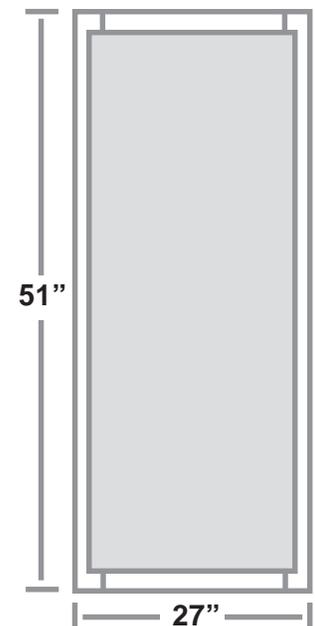
and nail the boards into place. Nail the side pieces onto the base frame. To complete the box, nail the ends onto the base and sides. To reinforce the box, place a nail at least every three inches wherever plywood and 2" x 4"s meet. Drill twelve 1/2" holes through the bottom of the box for drainage.
