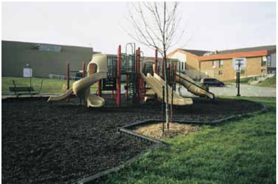
The St. James School in Liberty qualified for a Missouri Department of Natural Resources grant to install a playground utilizing crumb rubber as the cushioning play surface.
