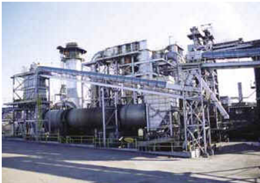
At Kingsford's Belle charcoal plant, sawdust is dried in the foreground drum. The retort chamber on the right converts it to charcoal while the after-combustion chamber stack on the left destroys smoke produced during the process.
