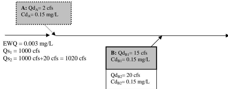
Note:  $Q_{S1}$  is the flow upstream of the affected segment (i.e., upstream of Plant A) and  $Q_{S2}$  is the flow downstream of Plant B after the consolidation/expansion.
