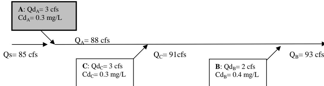
Note:  $Q_s$  is the 7Q10 stream flow.  $Q_A$ ,  $Q_B$ , and  $Q_C$  are the stream flows downstream of Plants A, B, and C, respectively (i.e., 7Q10 plus facility flows).
