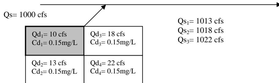
Note:  $Q_s$  is the 7Q10 stream flow.  $Q_{s1}$ ,  $Q_{s2}$ , and  $Q_{s3}$  are the stream flows (i.e., 7Q10 plus facility flow) downstream of the WWTF after the first, second, and third expansions, respectively.
