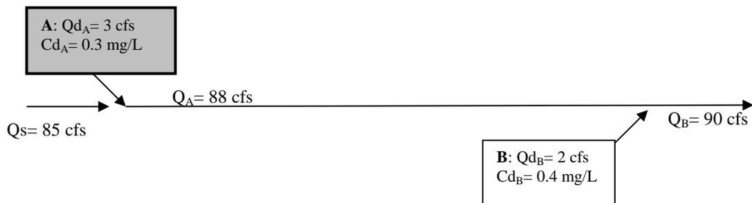
Note:  $Q_s$  is the 7Q10 stream flow.  $Q_A$  and  $Q_B$  are the stream flows downstream of Plants A and B, respectively (i.e., 7Q10 plus facility flows).
