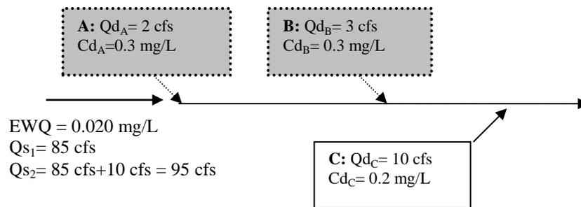
Note:  $Q_{s1}$  is the flow upstream of the affected segment (i.e., upstream of Plant A) and  $Q_{s2}$  is the flow downstream of Plant C after the consolidation.
